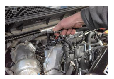
**STEP 3:** Disconnect the electrical connector from the MAP sensor by depressing the locking tab.
