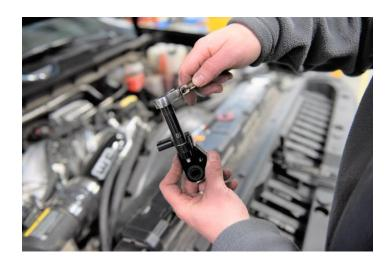
**STEP 6:** Clean the manifold surface of any debris and install the sensor block onto the original factory sensor location. Install the cap head bolt included in the kit and tighten it using a 5mm allen wrench. Reconnect the chassis harness electrical connector to the MAP sensor.
