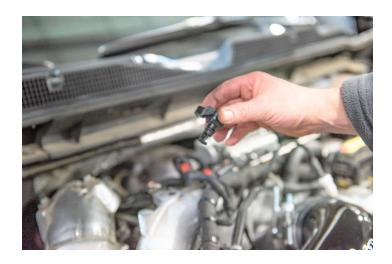
**STEP 5:** Install the MAP sensor into the Fleece Performance sensor block. Using the original fastener and 10mm socket, tighten the bolt to retain the sensor into the spacer block.
