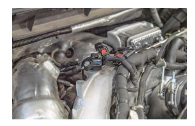
**STEP 2:** Loosen and remove the MAP sensor retaining bolt with a 10mm socket. The bolt will be reused to install the sensor into the new spacer block.
