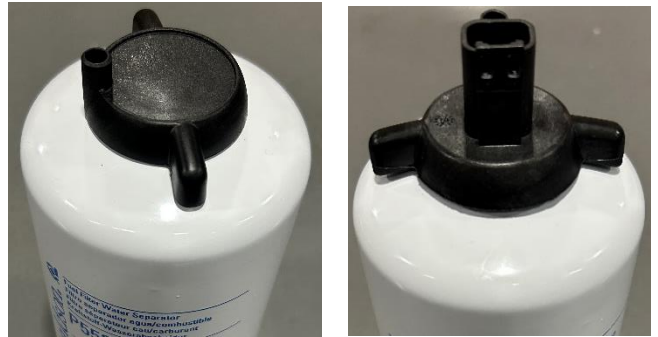
Figure 13: Donaldson fuel filter without WIF sensor (left), and Donaldson filter with WIF sensor installed (right).
