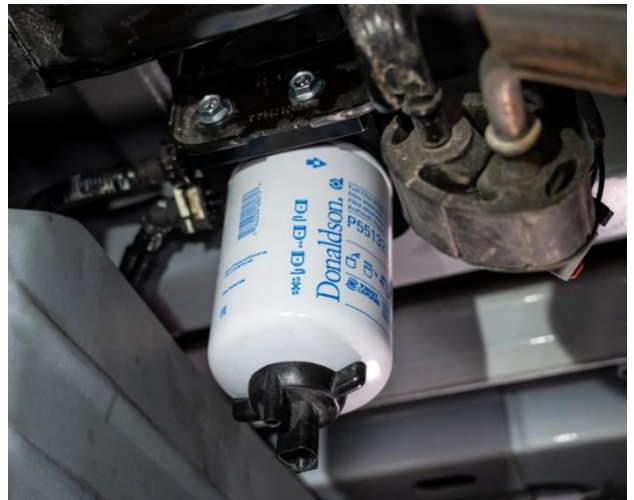
Figure 14: Donaldson fuel filter installed onto Fleece filter base.
