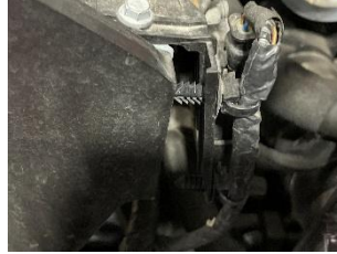
Figure 14: Fir Tree fasteners retaining wiring harness to passenger side battery tray.
