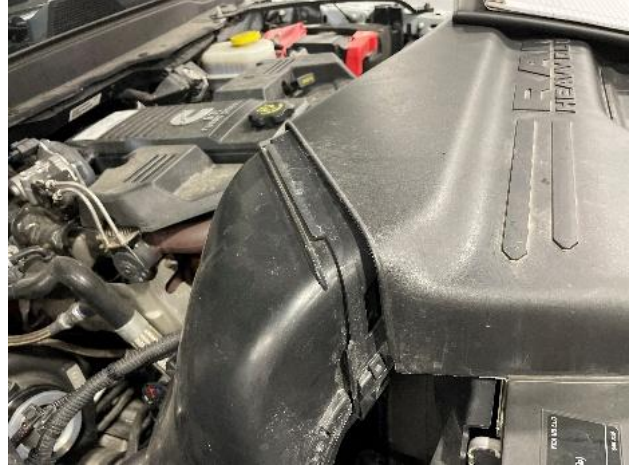
Figure 39: Plastic air inlet tube to the right of the engine air filter housing reinstalled.
