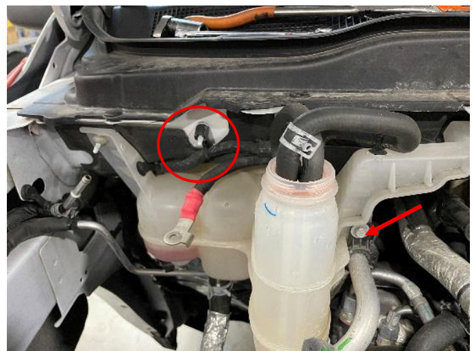
Figure 21: All coolant lines tucked into the stock coolant tank. Wiring harness retainer circled.
