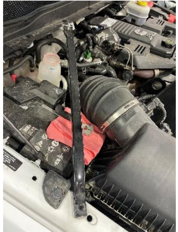
Figure 41: Passenger fender brace reinstalled in factory location.
