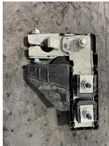
Figure 12: Positive terminal cluster removed.
