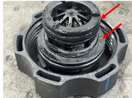
Figure 2: Coolant cap, O-rings highlighted with arrows.
