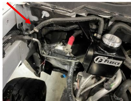
Figure 33: Installation of opposite end of coolant feed hose.
