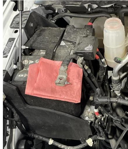
Figure 1: Negative terminal isolated with a shop rag.
