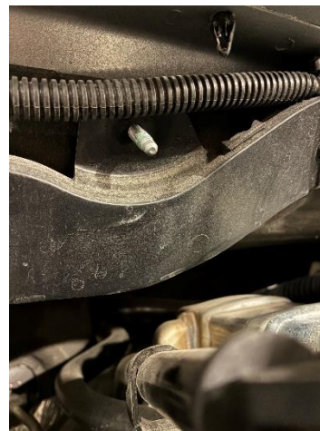
Figure 29: Original mounting studs for stock coolant tank, this location will not be used.
