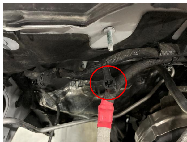
Figure 31: Previously unused stud at firewall. Wiring retainer circled.
