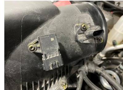
Figure 7: Barometric Pressure sensor (left) and MAF sensor (right) disconnected.
