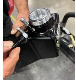
Figure 25: Thread sealant application on 1/8" NPT fitting.
