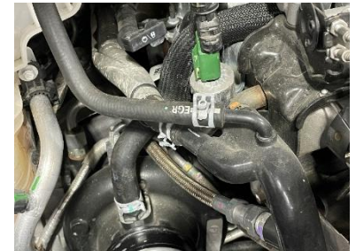
Figure 20: One of two coolant hose, attached at coolant standpipe.
