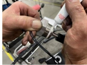
Figure 24: Thread sealant application on coolant level switch.
