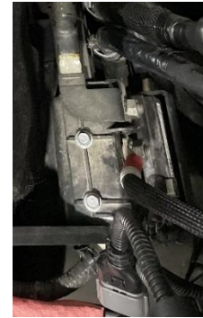
Figure 15: 8MM bolts retaining grid heater relay.
