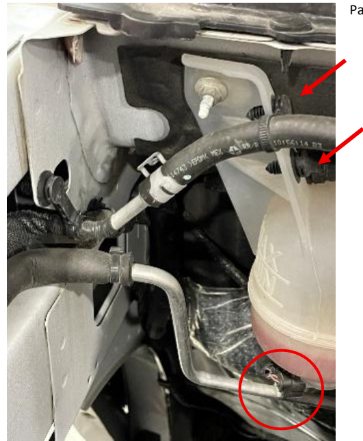
Figure 18: Coolant level sensor unplugged. Firtree fasteners highlighted with arrows.
