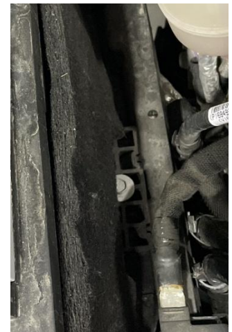
Figure 13: Battery hold down and 10MM retaining bolt.
