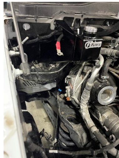
Figure 17: Battery tray removed.
