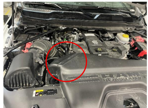
Figure 8: plastic air inlet tube to the right of the air filter housing.
