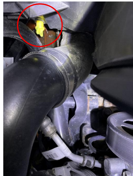
Figure 3: Radiator petcock in open position.
