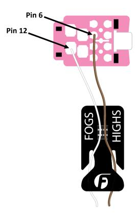
**STEP 6:** Position the ALL Lights On module so that it will not interfere with the connection when installed. Ensure that the wires are centered in the connector on the module.
