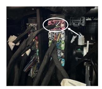
**STEP 3:** Using a sharp utility knife, CAREFULLY trim back 3 inches of the sheathing covering the harness. Cut the sheathing in the same direction that the wires are running to avoid any damage or knicks to the wires.
