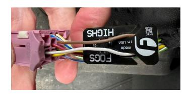
**STEP 7:** Place the connector cover over the two wires and squeeze it downward with a pair of pliers to force the wires into the insulation displacement prongs. Reinstall the pink connector back into the LCM.
