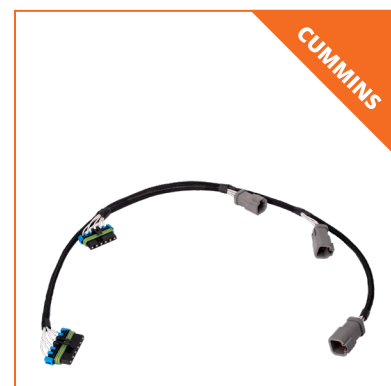
Valve Cover Conversion Harness (03-05 to 2006+) FPE-HAR-CUMM-VC-ADPT-EARLY
