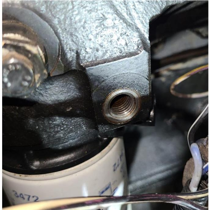
**STEP 5:** Install the new banjo fitting, 12mm banjo bolt and two, 12mm copper crush washers included in the kit onto the open port on the fuel filter housing.
