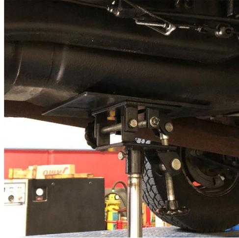
**STEP 5:** Remove 15 mm nuts that retain the fuel tank straps at the front and rear of the tank. Remove the tank straps.
