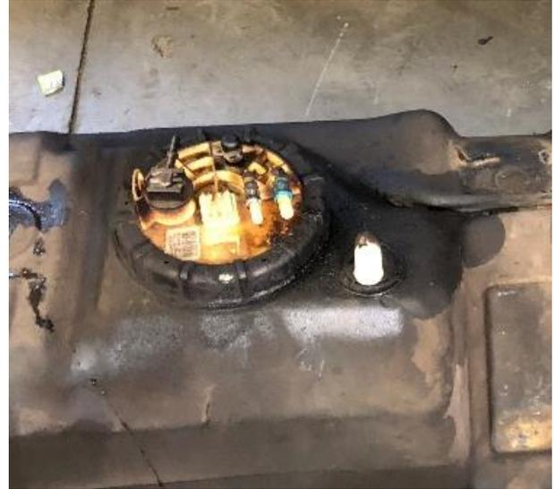
Using a strap wrench, or MATCO tool [#FTR730](#), rotate the sending unit's retaining ring (OE P/N: 52005389) counterclockwise. MATCO tool shown at right for reference. Remove the retaining ring and remove the sending unit assembly from the tank. Have a bucket nearby to catch fuel from the OE sending unit when removed.
