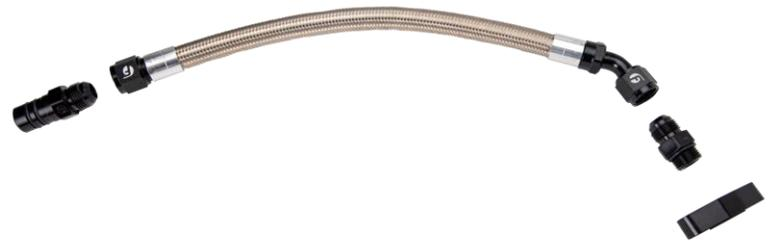
ENSURE THAT THE O-RING SIDE OF THE ADAPTER FITTING IS THREADED INTO THE TURBO FLANGE ADAPTER. THE FLARE SIDE OF THE ADAPTER FITTING WILL BE TOWARD THE DRAIN LINE. IF THE FITTING IS REVERSED, THE LINE WILL LEAK.
