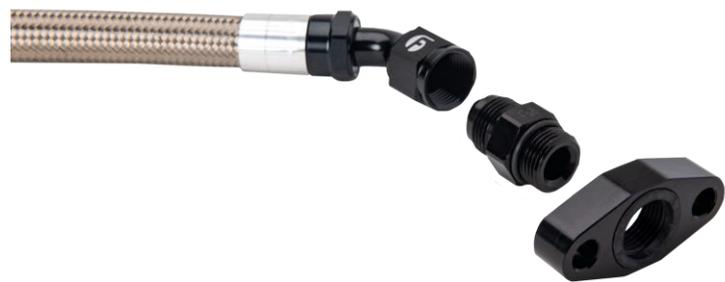
THOROUGHLY CLEAN THE BORE IN THE ENGINE BLOCK WITH SCOTCHBRITE PRIOR TO INSERTING THE DRAIN TUBE ADAPTER. LUBRICATE THE ORINGS AND FITTING LIGHTLY WITH GREASE PRIOR TO INSERTING.
