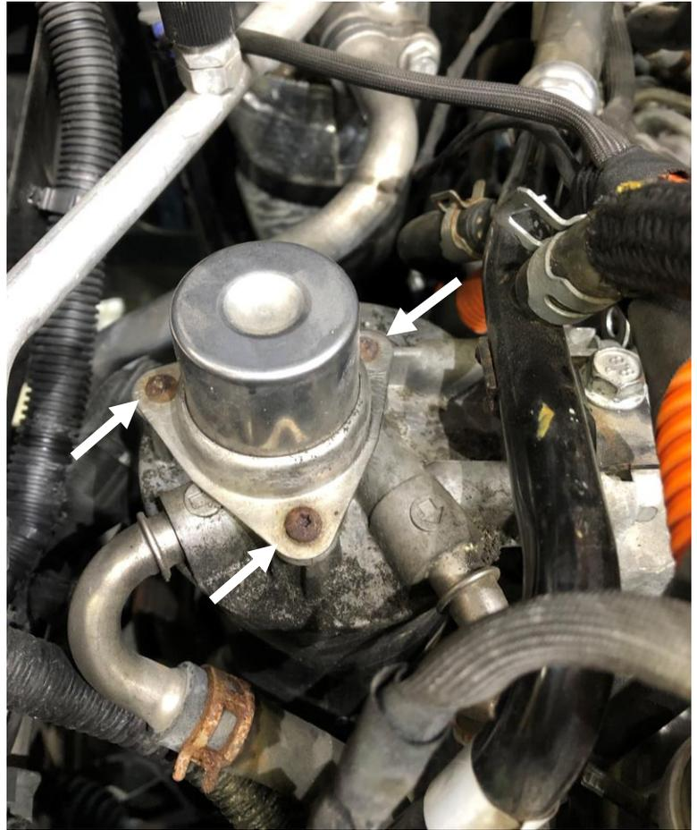
**STEP 2:** Remove all portions of the primer bulb from the top of filter head – these components can be discarded and will not be reused.
