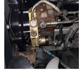
A fully installed 6.7L CP3 is shown at right.
