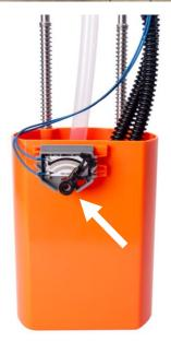
STEP 12: Install the SureFlo sending unit into the tank and reinstall the retaining ring using your hammer and punch or chisel by rotating it clockwise to the fully engaged position. Ensure proper orientation of the pump and fittings matches the orientation of the original unit.
