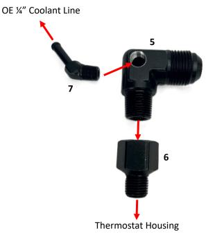
**STEP 6:** Install the 45-degree ¼" hose barb adapter (item 7) into the threaded hole on the side of item 5 using the included thread sealant. Align the fitting so that it is oriented towards the rear of the engine as shown at right.
