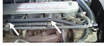
**STEP 16:** Connect the coolant bypass hose to the - 10AN 90 degree adapter and tighten the fitting.
