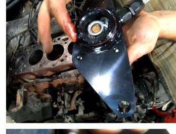
**STEP 12:** Slide the thermostat housing between the firewall and the back of the engine block. Align the thermostat housing with the original freeze plug hole location and press the housing against the engine to seat the housing. The coolant bypass hose should be oriented towards the passenger side of the vehicle and over the exhaust manifold.
