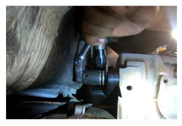
**STEP 14:** Fit the vinyl P-clamps (item 8) over the coolant bypass line and fasten the clamps to the coolant tubes running parallel to the engine using the supplied M8 fasteners (item 4).
