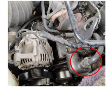
**STEP 4:** Install the 3/8" to %" NPT adapter (item 6) onto the thermostat housing. Use the included thread sealant to ensure a proper seal. Torque to 16 in-lbs.
