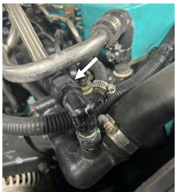
**STEP 17:** Ensure that the coolant drain plug has been reinstalled in the radiator and proceed to re-fill the coolant system. Re-use or replace coolant as necessary to properly fill the system with clean fluid.
