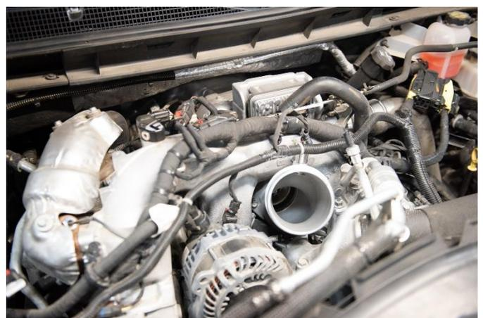
**STEP 10:** Reinstall the AC compressor using the four 15mm bolts removed in step 5. Torque to 43 ft-lbs.
