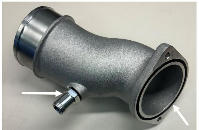
**STEP 9:** Install the new intake horn with the included bolts using a 13mm socket. Be sure that the mating surfaces on the turbocharger and intake horn are clean and free of any contamination before installation. Torque the bolts to 18 ft-lbs.
