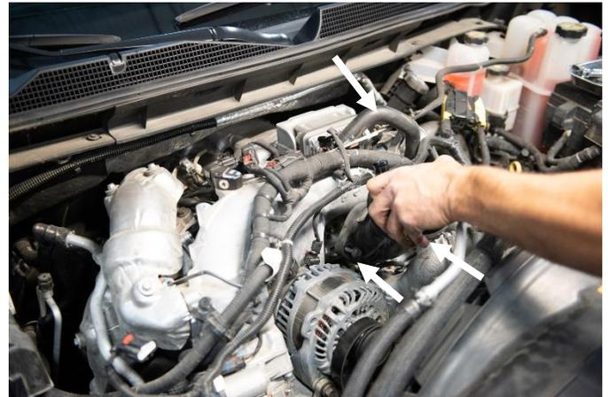
**STEP 7:** Remove the two bolts connecting the intake horn to the turbo compressor housing using a 13mm socket and remove the OE intake horn. Discard the original intake horn o-ring.
