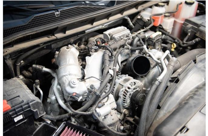
**STEP 3:** Remove the two nuts that retain the AC harness bracket on top of the AC compressor using a 13mm socket. Remove the bracket.
