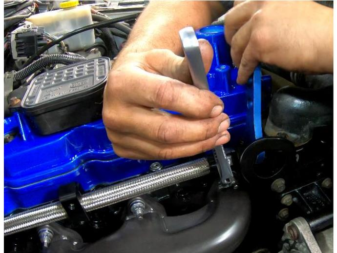
**STEP 13:** Utilizing the coolant bypass hose brackets and M8 socket head cap screws in your kit; position the clamps over the bypass coolant hose and fasten them to the cylinder head in the available tapped holes between cylinder numbers 2 & 3 as well as between cylinder numbers 4 & 5.
