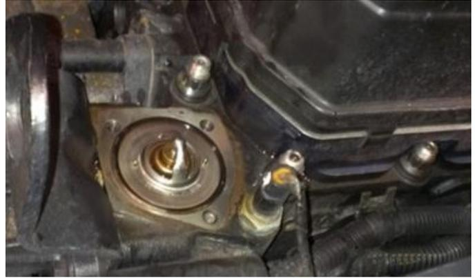
**STEP 4:** Remove the stock thermostat. Inspect it for wear and proper function. Using a Scotch-Brite™ pad and degreasing solution, thoroughly clean the sealing surface of the stock thermostat and thermostat housing. Be sure to remove any foreign debris.
