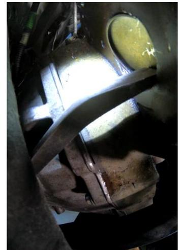
**STEP 7:** With the freeze plug removed, use a Scotch-Brite™ pad and a degreasing solution to **THOROUGHLY** clean the block surface area from the head down to the rear cover, as well as the bore where the freeze plug was previously installed. Be sure to remove all dirt and foreign debris to allow the coolant bypass thermostat housing to fully seat.
