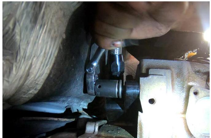
**STEP 12:** Route the coolant bypass hose above the exhaust manifold and thread the hose fitting onto the coolant riser block fitting. Using a backup wrench, tighten the fitting.
