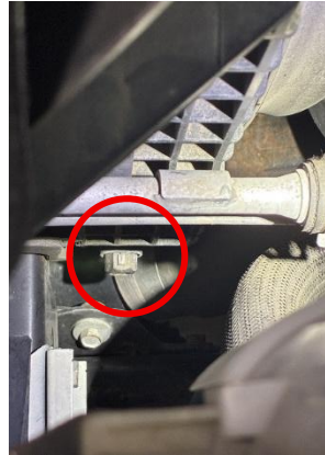
Figure 9A: Coolant drain turned to close position.
