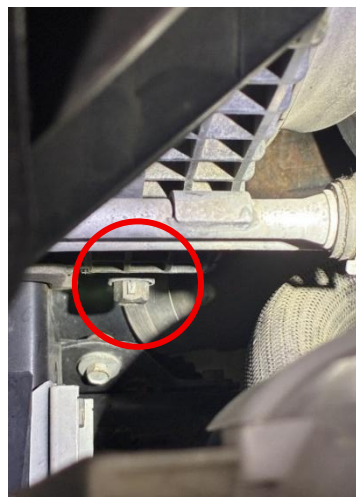
Figure 3A: Radiator coolant drain turned to the open position, model years 2013-2024.
