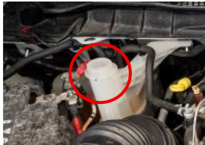
Figure 2A: Coolant overflow cap.
