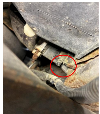
Figure 3B: Radiator coolant drain, model years 2003-2012.
