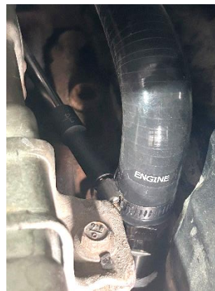
Figure 8A: Installation of supplied hose clamp at cylinder head.
