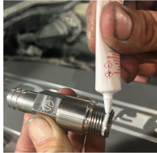
Figure 6: Application of thread sealant on heater core hose riser fitting.
