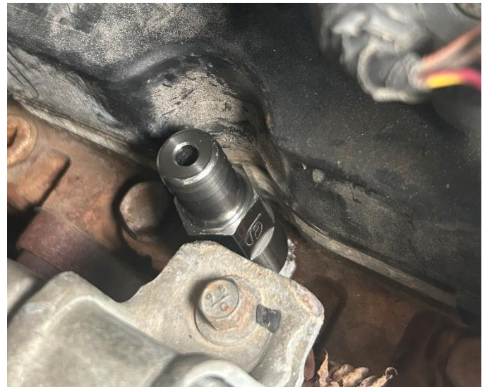
Figure 7: Installation of heater core hose riser fitting.
