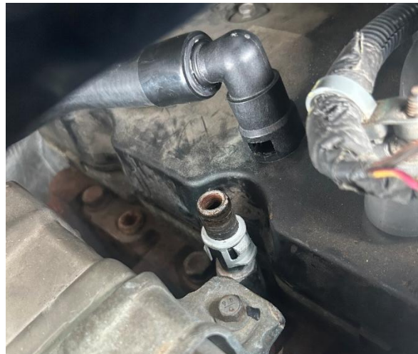
Figure 5: Heater hose disconnected from OE adapter fitting.
