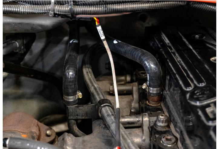
Figure 6: New Fleece heater core lines installed, supplied hose clamps installed.
