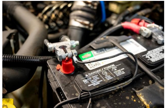
Figure 1: Negative battery terminal disconnected and isolated.
