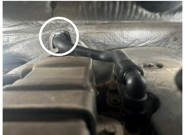
Figure 4: Heater hose clamp at firewall.
