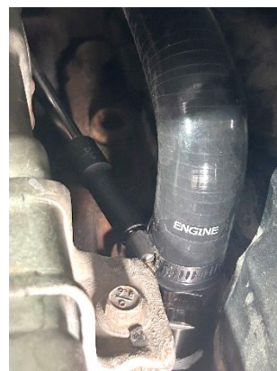
Figure 11A: Installation of supplied hose clamp at cylinder head.
