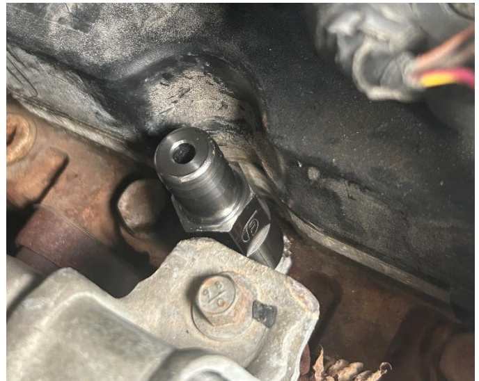
Figure 10: Installation of heater core hose riser fitting.
