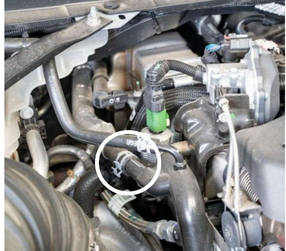
Figure 6: Heater core return hose, clamp circled at standpipe.
