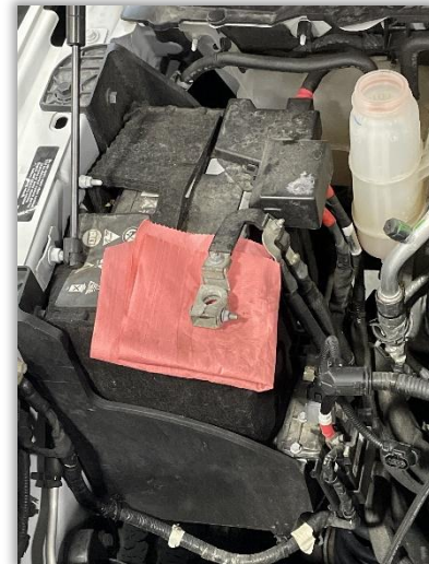
Figure 1: Use of shop towel to isolate negative terminal.
