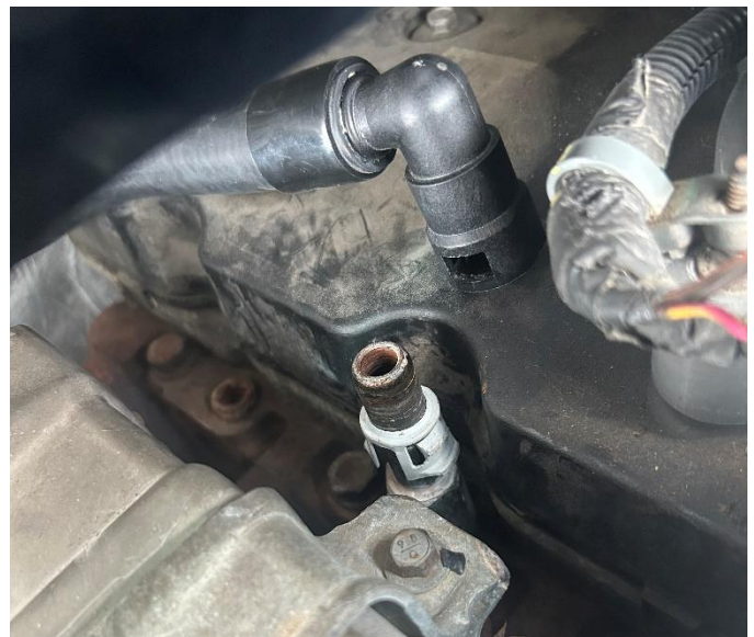
Figure 5: Heater hose disconnected from OE adapter fitting.
