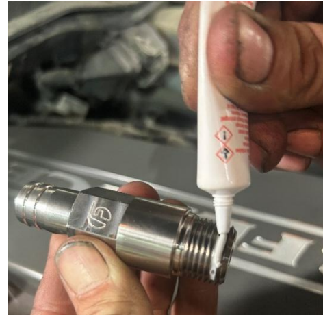
Figure 9: Application of thread sealant on heater core hose riser fitting.
