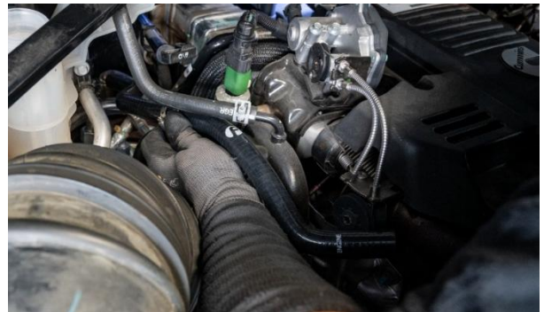
Figure 7: Installation of New Fleece Performance lower heater hose.
