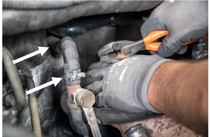
Figure 4: Stock heater core return hose. Clamps highlighted with arrows.
