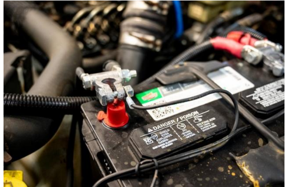
Figure 1: Negative battery terminal disconnected and isolated.
