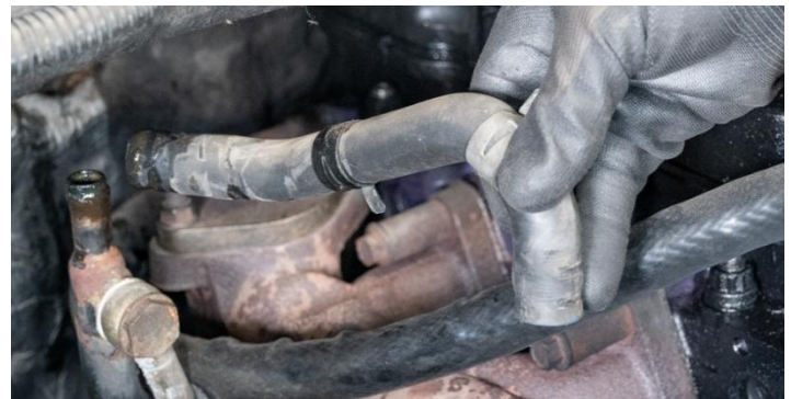
Figure 5: Removal of stock heater core return hose.
