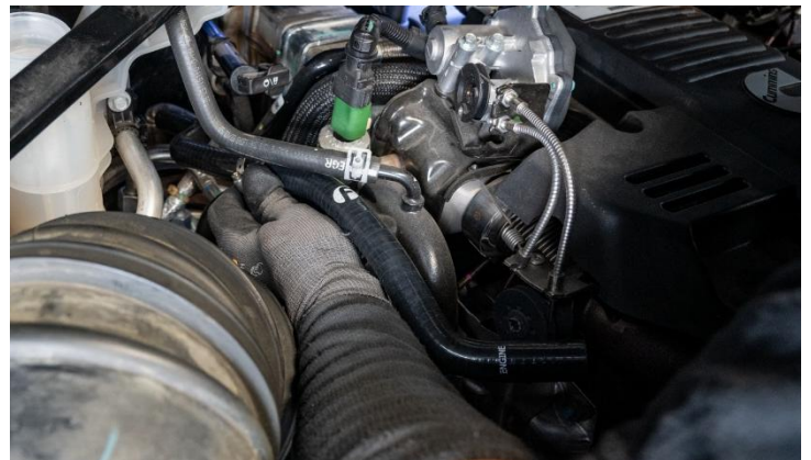
Figure 5: Installation of New Fleece Performance lower heater hose.
