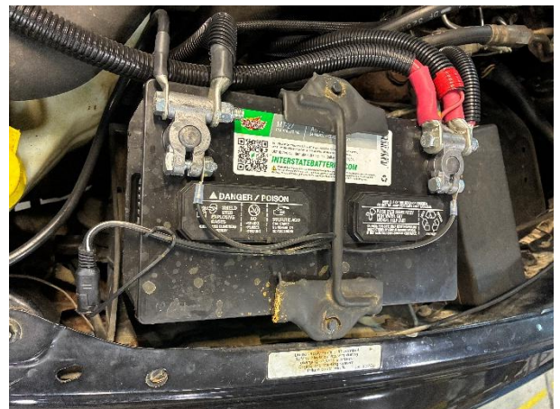
Figure 14: Negative battery terminal reinstalled.
