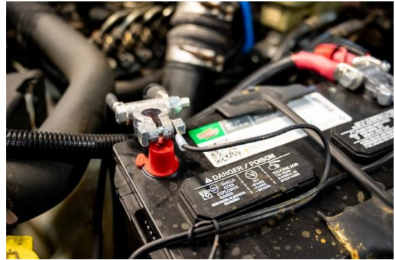
Figure 1: Negative battery terminal disconnected and isolated.
