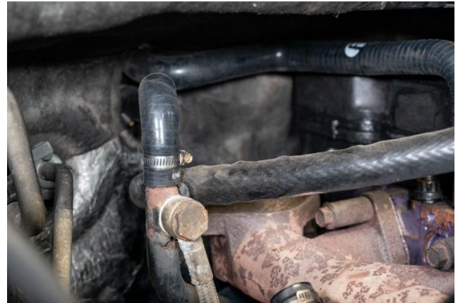
Figure 8: New Fleece heater core line installed, included hose clamps installed.
