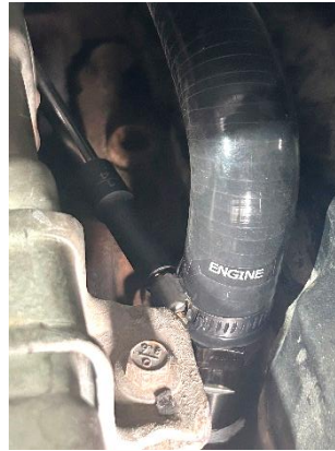
Figure 11: New Fleece heater core line installed, included hose clamp installed.
