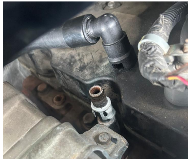
Figure 5: Stock heater core hose and OE adapter fitting.
