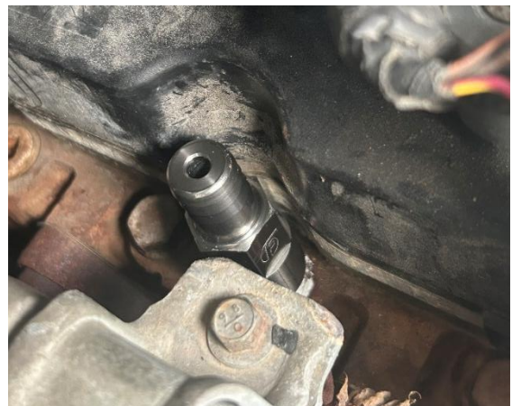
Figure 10: New Fleece heater core line installed, included hose clamp installed.
