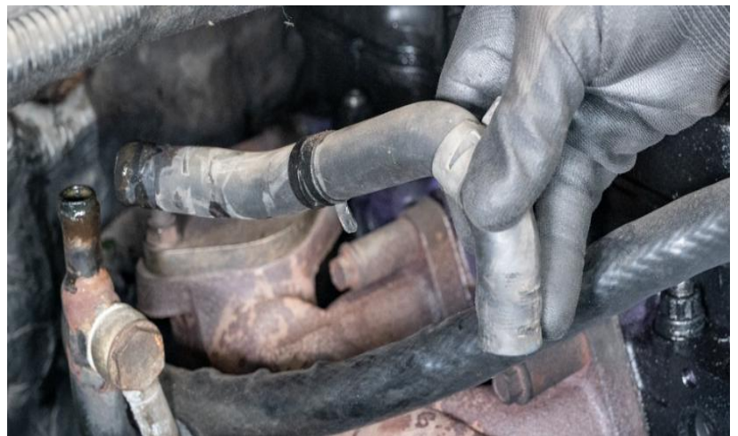
Figure 7: Removal of lower heater core return hose.
