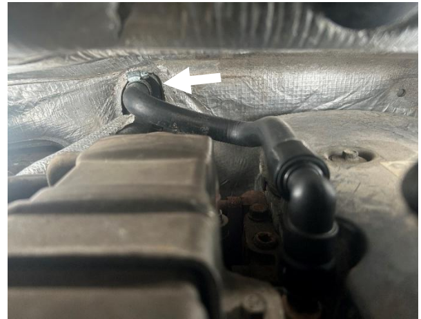
Figure 4: Upper heater core supply hose, hose clamp highlighted with arrow.
