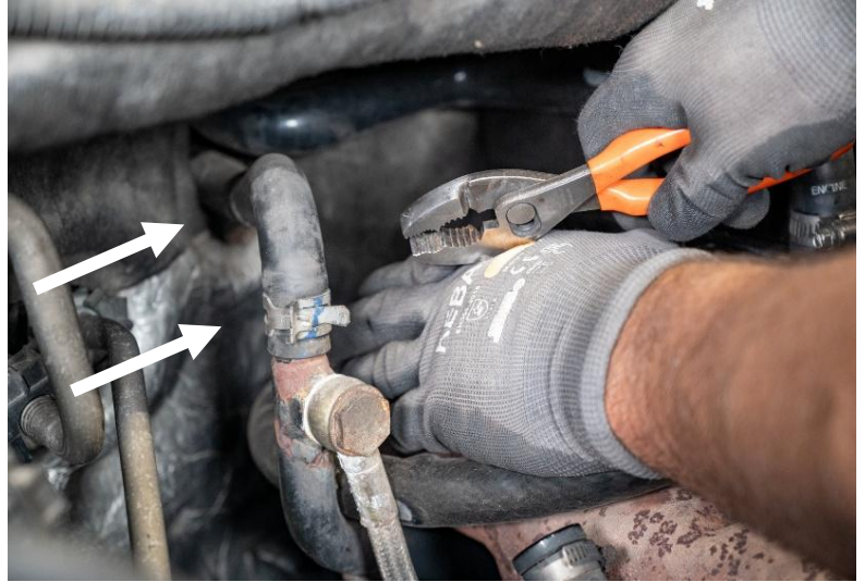
Figure 6: Stock lower heater core return hose. Arrows highlighting each clamp.
