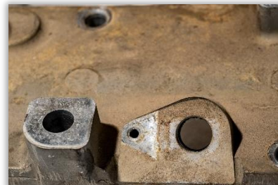
Figure 8A: Map sensor Location on intake plenum.
