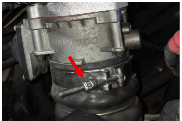
Figure 5: Throttle valve with CAC boot attached.
