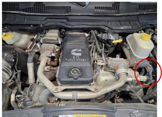
Figure 2: Engine cover removed. EGR valve connector is circled. The EGR temp sensor is pictured off to the left of it.
