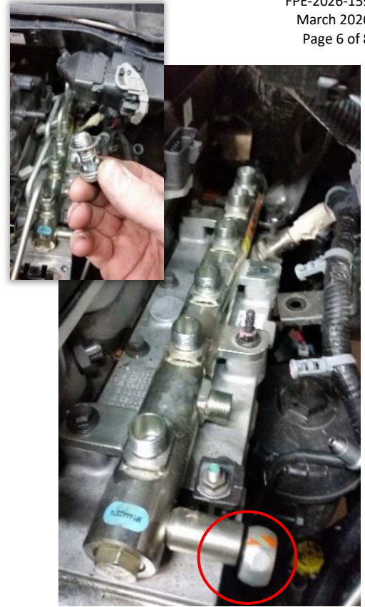
Figure 11: Injection lines removed, fuel return line circled.
