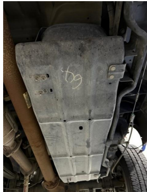
Figure 23: SureFlo installed, Skid plate reinstalled.
