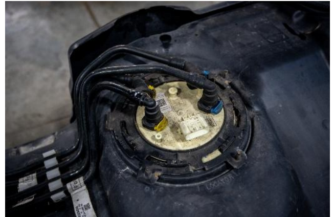
Figure 9: Fuel tank removed, top of stock lift pump.
