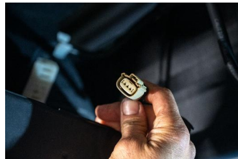
Figure 6: WIF sensor connector disconnected.
