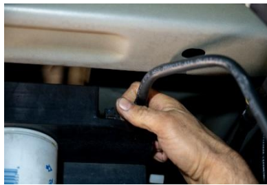
Figure 4: Removal of fuel return line.
