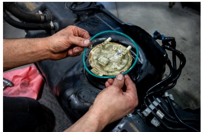
Figure 11: Removal of stock lift pump, removal of old sealing O-ring on top of the fuel tank.
