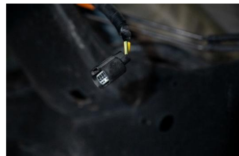
Figure 8: Stock lift pump electrical harness disconnected.
