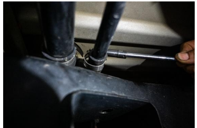
Figure 3: Hose clamps retaining the fuel filler tube (left) and fuel tank vent (right).
