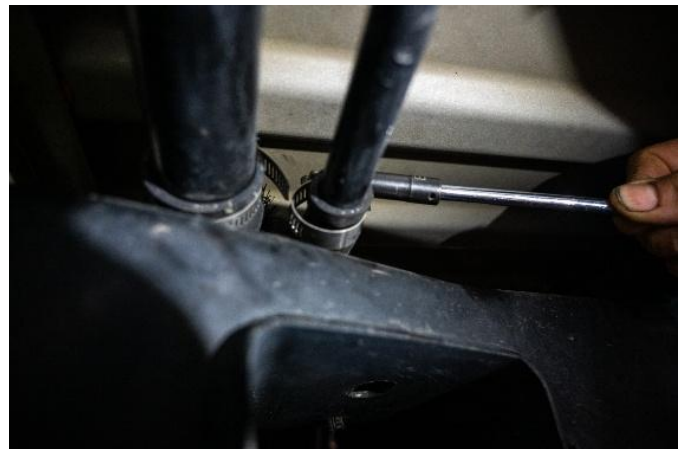
Figure 21: Fuel filler tube and fuel breather tube reinstalled.
