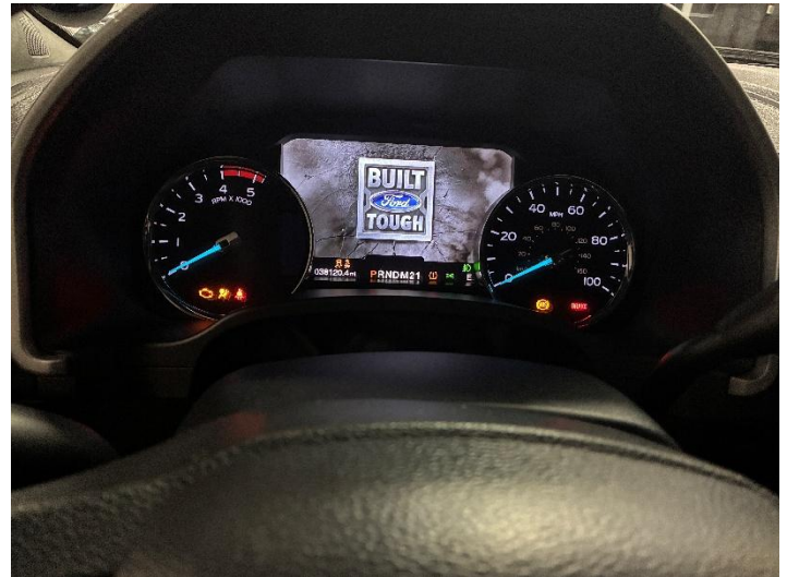
Figure 22: Ignition in "run" position. Lights on dashboard illuminated, engine off. Verify the fuel level is being displayed correctly.
