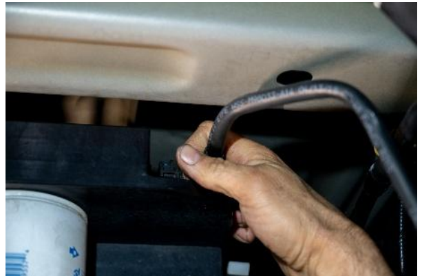
Figure 19: Reinstallation of fuel return line.
