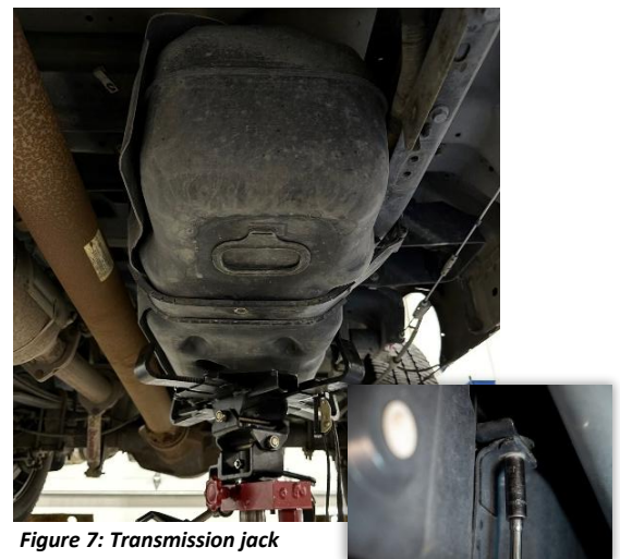
Figure 6: WIF sensor connector disconnected.
