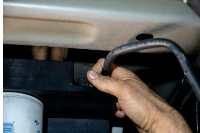
Figure 20: Reinstallation of fuel return line.
