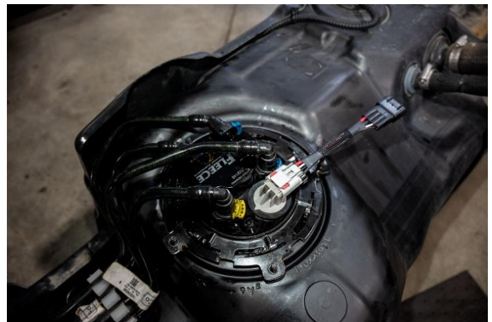
Figure 17: Fuel lines installed and extension harness plugged in at top of PowerFlo.
