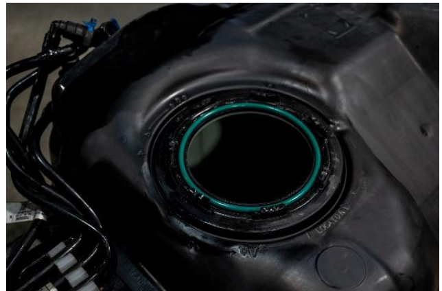
Figure 12: Cleaned and inspected fuel tank, new sealing O-ring installed.
