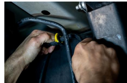
Figure 5: Removal of fuel return line.
