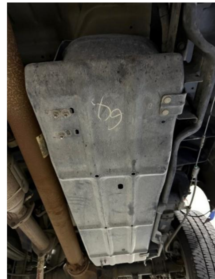
Figure 2: Skid plate attached to underside of the fuel tank.
