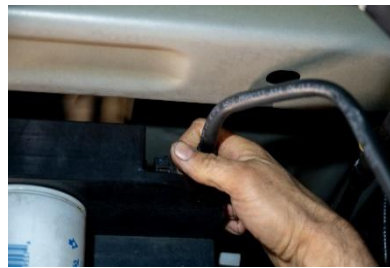
Figure 4: Removal of fuel feed line.
