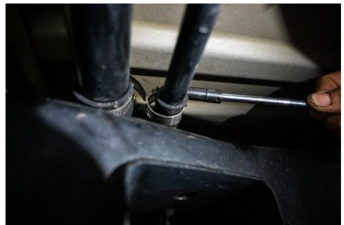
Figure 3: Hose clamps retaining the fuel filler tube (left) and fuel tank vent (right).
