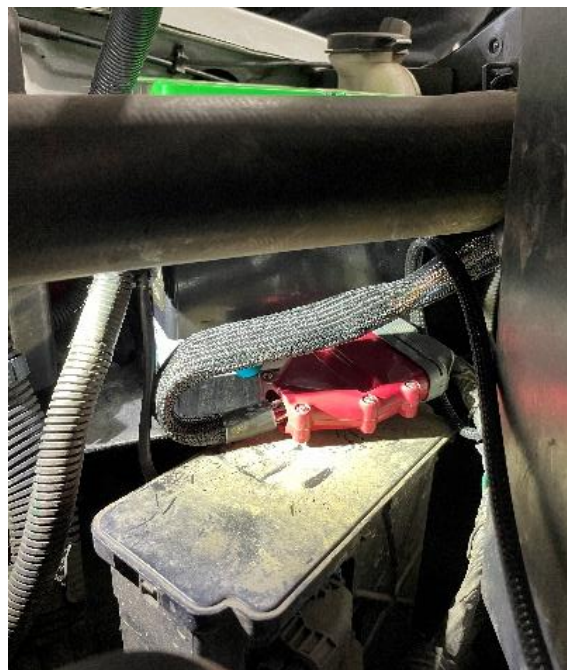
Figure 5: (J3) Connector installed into (J2) connector from the truck side harness.
