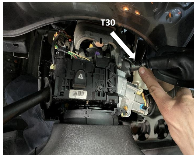
Figure 9: T30 Bolt retaining shift level, labeled for clarity.
