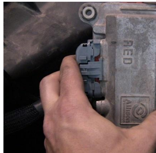
Figure 4: (J4) Connector installed into the red J2 connector on the TCM.
