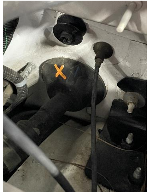
Figure 6: Factory Bulkhead. Incision can be made in rubber boot to route Tapshifter harness.
