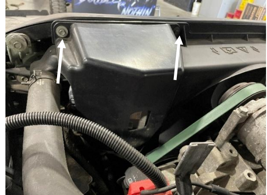
Figure 1: TCM Shroud, retaining bolts highlighted with arrows.
