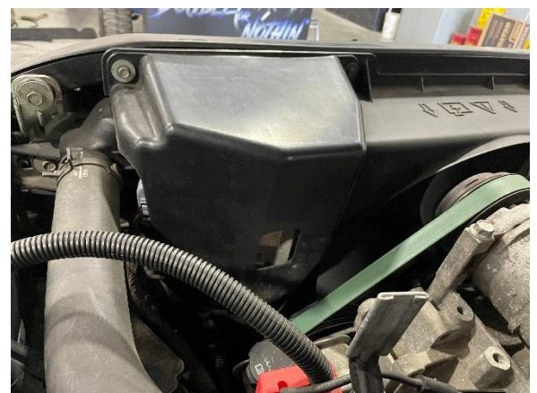
Figure 16: TCM shroud reinstalled.
