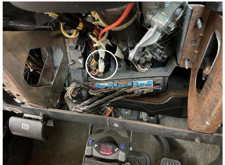
Figure 11: Four pin connector plugged into tapshifter harness. Circled for clarity.
