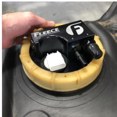
*NOTE: Use caution when installing the pump to not damage the float arm. When tightening the retaining ring, DO NOT allow the pump cap to rotate once the pump is installed in the tank, you will damage the float arm or sending unit if the flange rotates when the retaining ring is tightened.*
