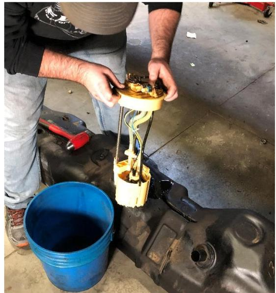
STEP 8: Remove the original gasket from the tank.
