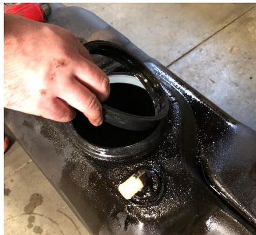
STEP 9: Install the new gasket included in the kit into the fuel tank. Clean the original retaining ring of debris and prepare it for re-use onto the new PowerFlo pump.
