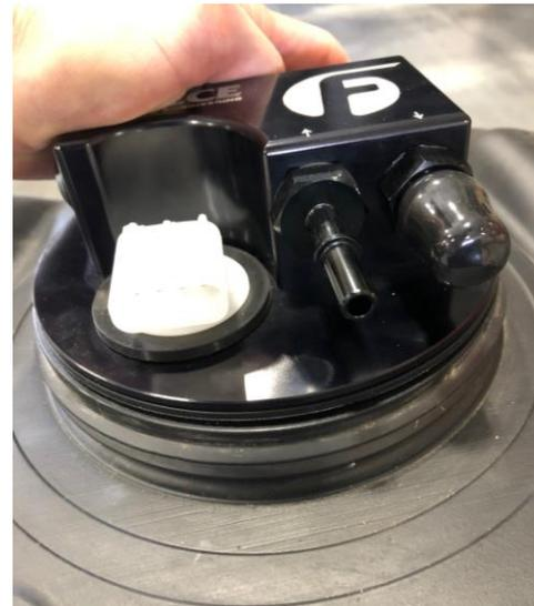
STEP 12: Reinstall the retaining ring using your hammer and punch or a strap wrench by rotating it clockwise to the fully engaged position. Ensure proper orientation of the pump and fitting by matching the orientation of the original sending unit.
