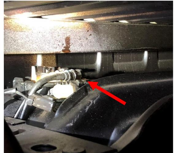
STEP 3: Remove the cross-member located at the front of the fuel tank. There will be 4, 15mm bolts to remove.
