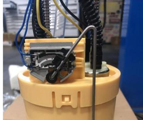
STEP 11: Install the PowerFlo pump assembly into the tank. Check that the gasket is fully seated.
