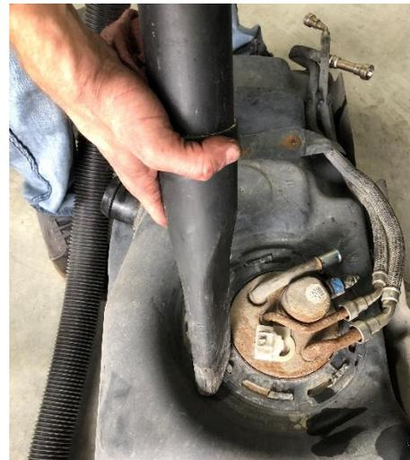
STEP 6: Remove the fuel line quick disconnects from the sending unit using a 1/2" and 3/8" fuel line disconnect tool.
