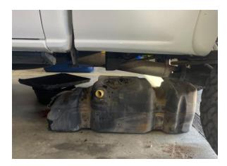
**STEP 6:** Thoroughly clean off the top side of the tank around the sending unit to avoid getting any debris inside the fuel tank when the sending unit is removed.
