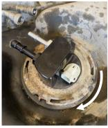
**STEP 14:** Reconnect the fuel lines to the lift pump feed and return quick disconnect fittings. Connect the new wiring harness supplied with the lift pump to the original OEM harness connector and the other end to the PowerFlo lift pump.
