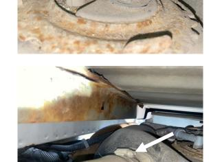
**STEP 4:** Remove the fuel lines at the front of the tank, and at the fuel cooler with a 3/8" and 1/2" fuel line disconnect tool.
