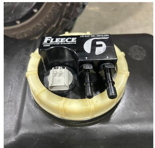
**STEP 13:** Remove the protective shipping caps from the fittings and install the new fuel line locking tabs that are included in your kit onto the return side fitting.
