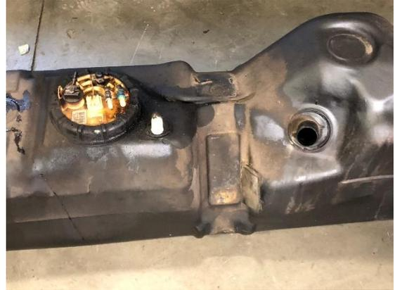
Using a strap wrench, Lisle 63000, or MATCO tool #FTR730, rotate the sending unit's retaining ring (OE P/N: 52005389) counterclockwise. MATCO tool shown at right for reference.
