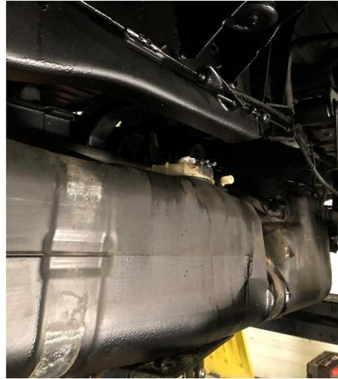
**STEP 16:** From the driver's side rear wheel-well, connect the electrical wiring harness to the SureFlo lift pump connector. Key on the vehicle and ensure the fuel level is reading appropriately. Start the engine and check for any fuel leaks before operating the vehicle.
