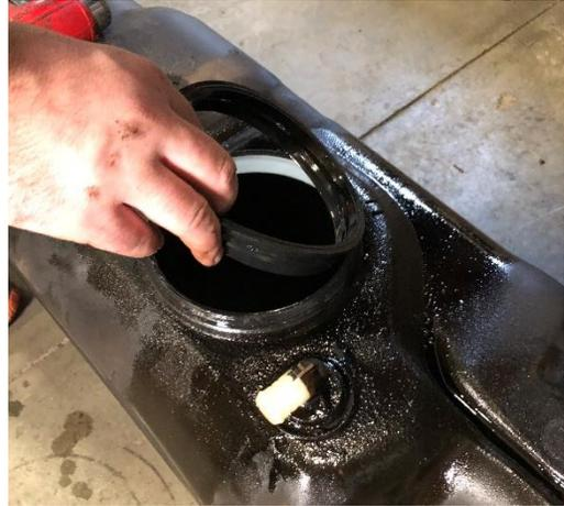
**STEP 9:** Install the new seal ring included in the kit onto the fuel tank. Clean the original retaining ring of debris and prepare it for re-use onto the new SureFlo sending unit.
