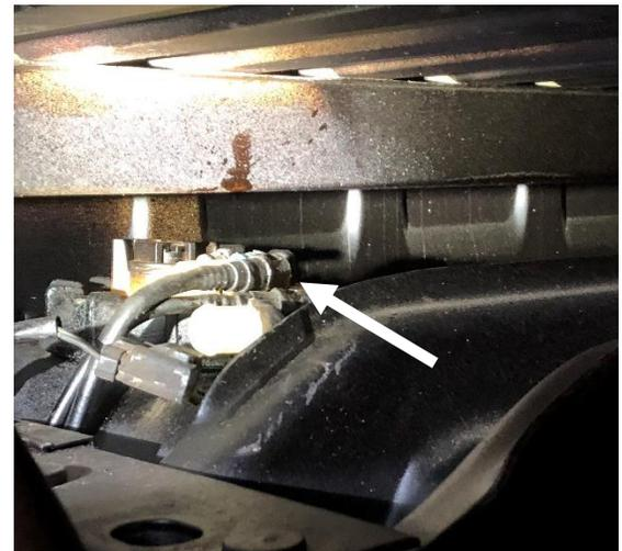
**STEP 3:** If present on your application, remove the cross-member located at the front of the fuel tank. There will be four 15mm bolts to remove.
