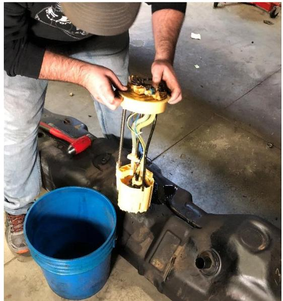
**STEP 8:** Remove and discard the original seal ring from the tank.
