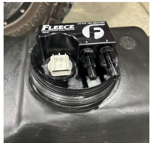
**STEP 12:** Ensure proper orientation of the SureFlo by matching the orientation of the original sending unit. Reinstall the retaining ring and tighten using a Lisle 63000, MATCO #FTR730, or a strap wrench by rotating it clockwise to the fully engaged position.
