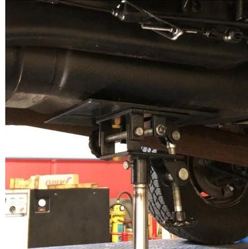
**STEP 5:** Remove the 15 mm nuts that retain the fuel tank hanger brackets at the front and rear of the tank. Remove the hangers.
