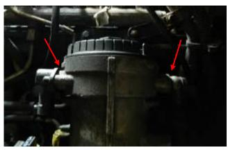
STEP 7: Use a 10mm socket to remove the two fuel filter assembly bolts that secure the assembly to the side of the head.
