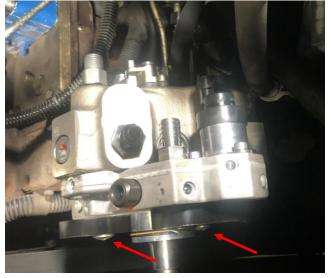
STEP 16: Locate the %" pushlock hose you installed to the distribution block in STEP 12 and route it neatly alongside the engine and up to the  $2^{nd}$  pump. Cut it to length and install it onto your FPE high flow feed fitting. Using the -6AN 120 degree fitting thread it onto the return side of your  $2^{nd}$  pump and neatly route the %" pushlock hose you installed to the AUX port of the distribution block, cut it to fit and install the remaining -6AN 90 degree fitting.
