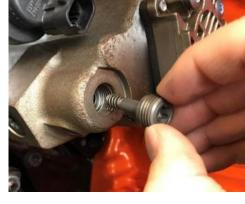
STEP 6.2: Ensure the check ball remains seated in place and does not fall out.
