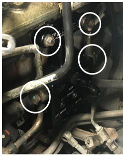
**STEP 11:** Install an M12 to -8AN fitting into the OEM low pressure feed of the factory CP3, route it using the two -8AN 90 degree fittings to the bottom front feed fitting on the distribution block as shown.
