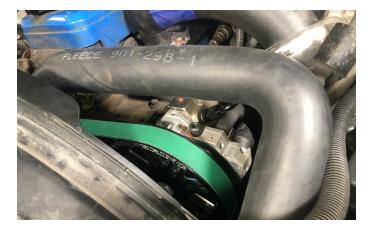
**STEP 21:** Install the new Fleece upper radiator hose using the OE clamps from the factory hose. Tighten the radiator drain and refill the cooling system at this time.
