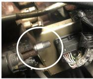
**STEP 6.1:** Remove plug with a T50 Torx bit.
