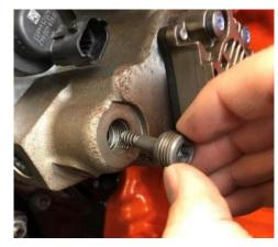
**STEP 6.2:** Ensure the check ball remains seated in place and does not fall out.
