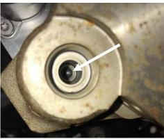
**STEP 6.3:** Remove the spring from the plug and reinstall onto the high-pressure CP3 fitting.
