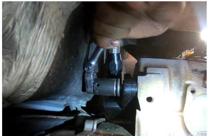
**STEP 12:** Route the coolant bypass hose above the exhaust manifold and thread the hose fitting onto the coolant riser block fitting. Using a backup wrench, tighten the fitting.
