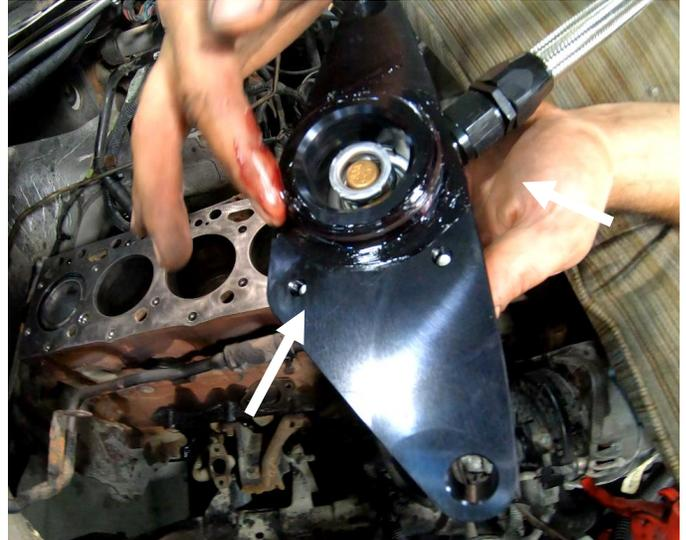
**STEP 10:** Slide the thermostat housing between the firewall and the back of the engine block. Align the thermostat housing with the original freeze plug hole location and press the housing against the engine to seat the housing. The coolant bypass hose should be oriented towards the passenger side of the vehicle and over the exhaust manifold.
