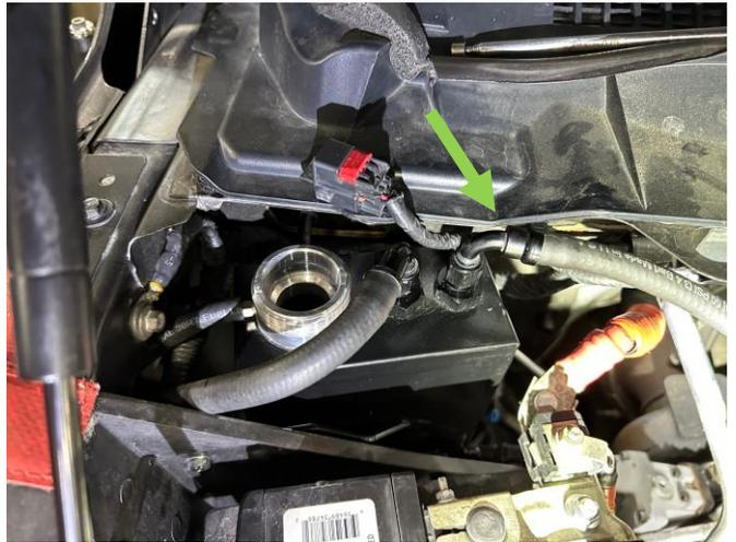
STEP 9: Using the -6AN 90 deg pushlock fitting included in the kit, attach this to the degas line that was disconnected from the OE coolant tank. It may be necessary to trim a small amount of hose to achieve a uniform routing along the left side of the tank.
