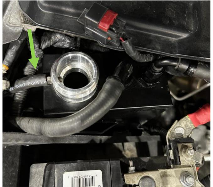
STEP 11: Install the -12AN 90 degree fitting onto one end of the new 3/4" heater hose included in the kit. Secure the hose to the fitting with one of the hose clamps included in the kit. Slide the heat wrap removed from the OE coolant hose over the new 3/4" hose.
