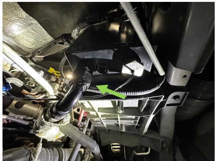
STEP 14: Connect the coolant level sensor to the factory harness that was disconnected during removal of the OE tank.
