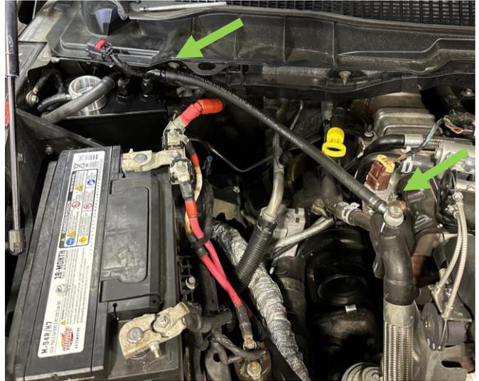
STEP 8: Connect the 90 degree -6AN fitting and hose that routes to the coolant riser pipe to the right side -6AN fitting on the coolant tank.
