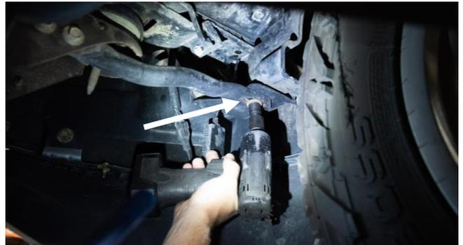
**STEP 7:** Remove the front bumper assembly to provide for clear access to the transmission oil cooler.
