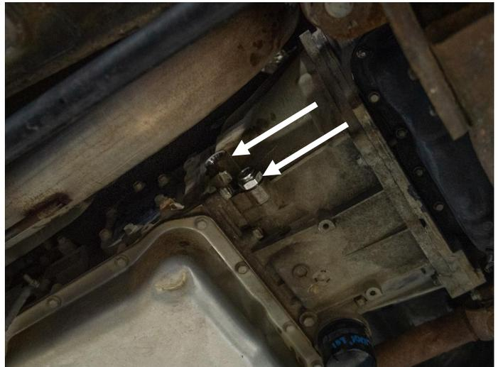
**STEP 16:** Install two of the 7/8"-14 O-ring to -10AN fittings into the "To Cooler" and "From Cooler" ports on the transmission
