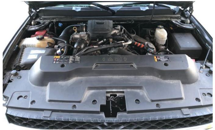
**STEP 2:** Remove the engine bay plastic cover panel by removing the plastic expansion fasteners that retain it to the front grill and body. Remove the front grill retention bolts located along the top of the grill.
