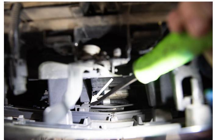
**STEP 4:** Remove the bumper by removing the upper retaining bolts with an 18mm socket.
