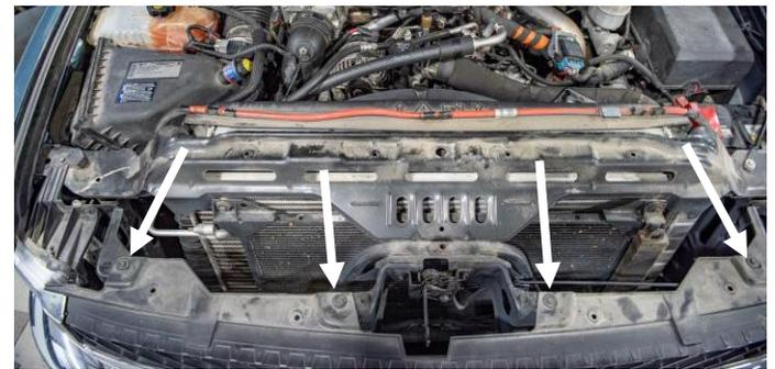
**STEP 3:** Using a long pry bar, release the lower retaining clips for the front grill. Remove the grill.
