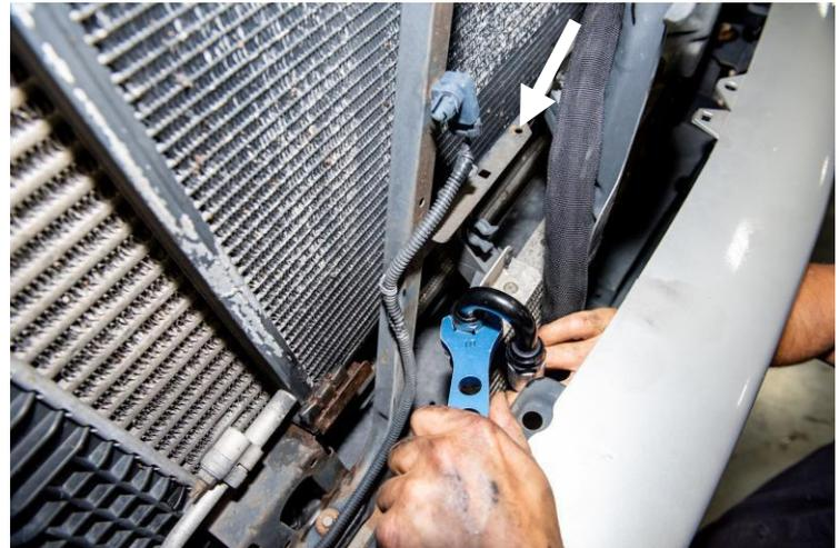
Route the lines over the top of the chassis cross-tube. Use the double hose clamps provided in the kit to secure the hoses together.
