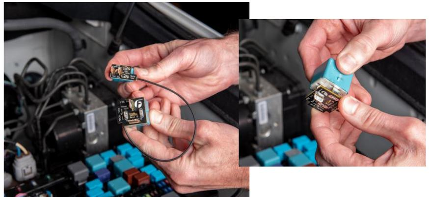
**STEP 4:** Reinstall the two relays back into their original location. Route the connecting wire along the side of the relay box. Install the relay panel cover.
